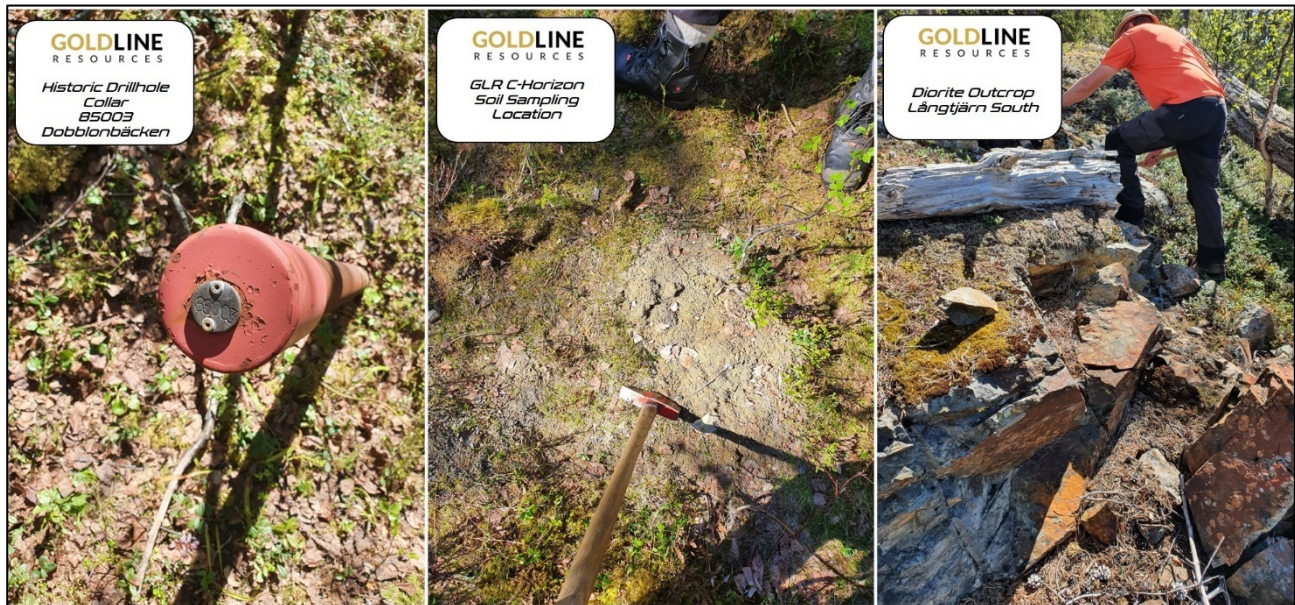
Figure 29: Photographs from the site visit to the Långtjärn property; historic drillhole collar (85003, Dobblonbäcken), GLR/EMSAB C-Horizon soil sampling site and outcropping diorite from Långtjärn South. (Source: SGAB).
