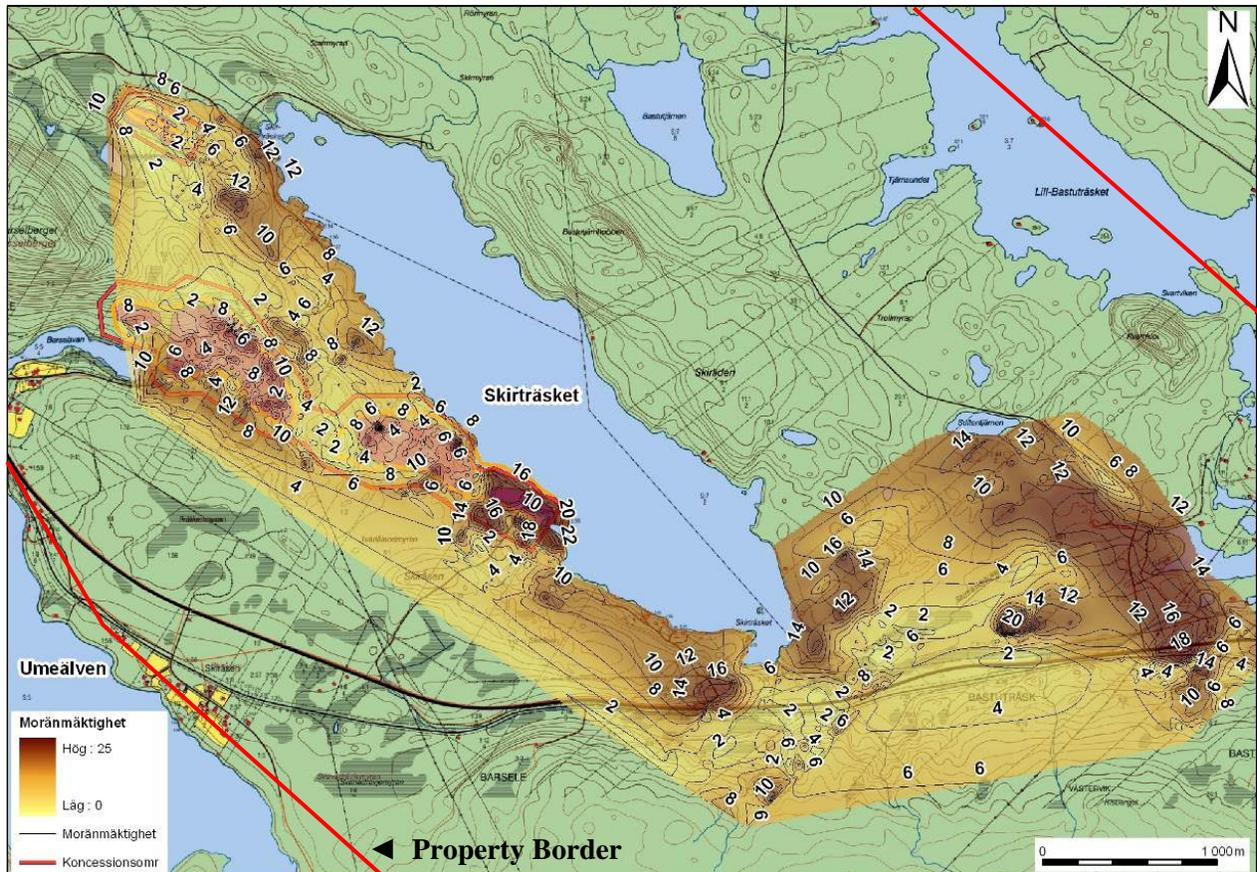
**Figure 5.1 - Depth of Glacial Till Cover (in meters)**
