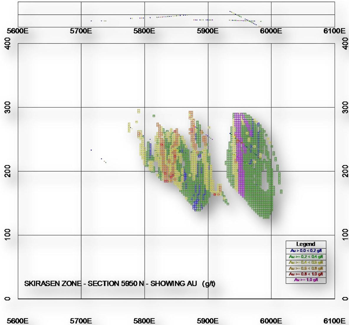
Figure 17.10: Skiråsen CrossSection 5950N Showing Au in Blocks & Composites
