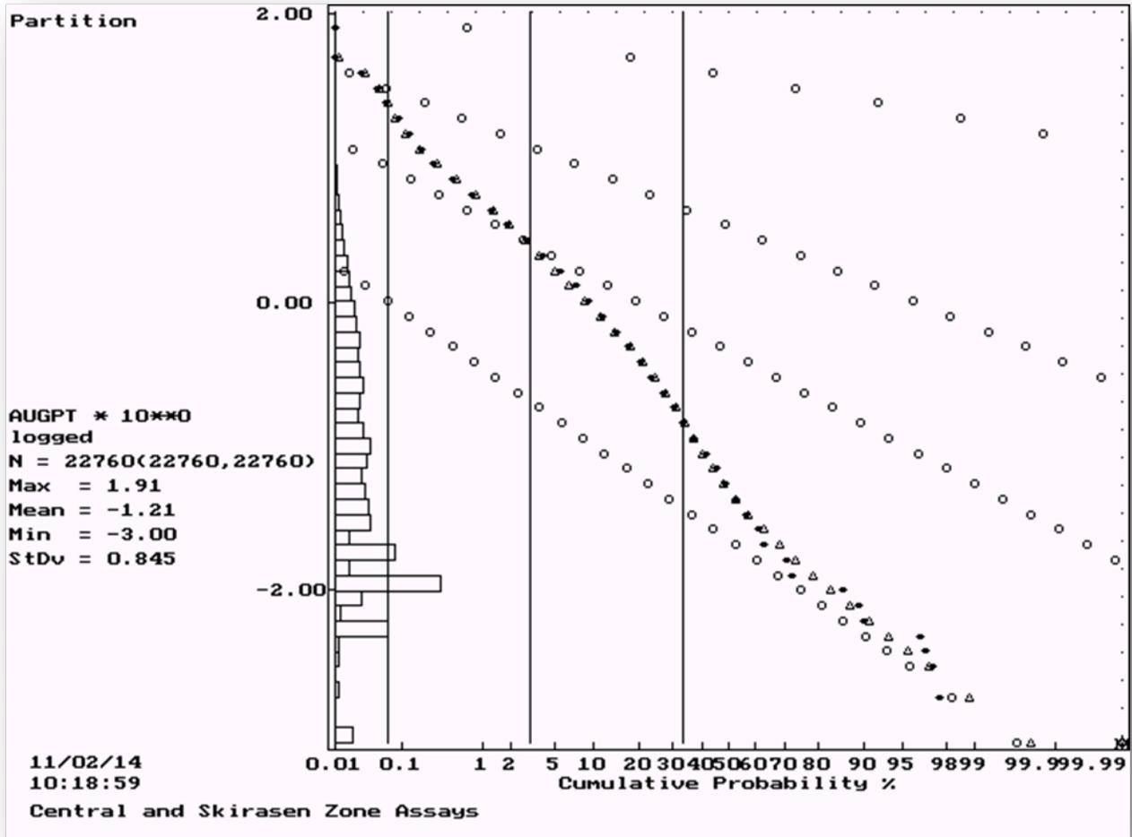
Figure 17.4: Lognormal cumulative frequency plot for Au in the Central & Skiråsen Zones
