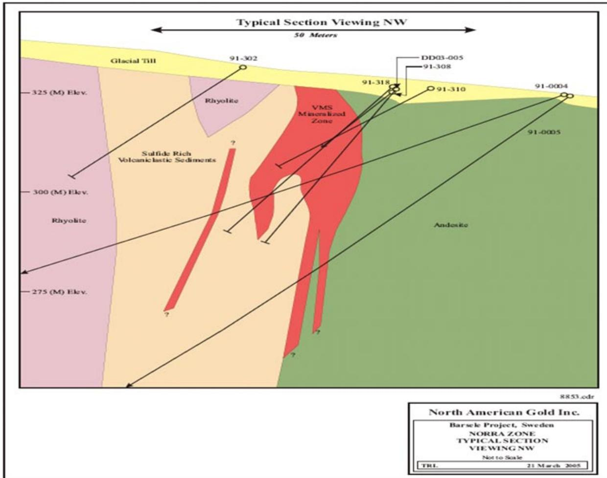
**Figure 9.2- Typical Norra Cross Section**
