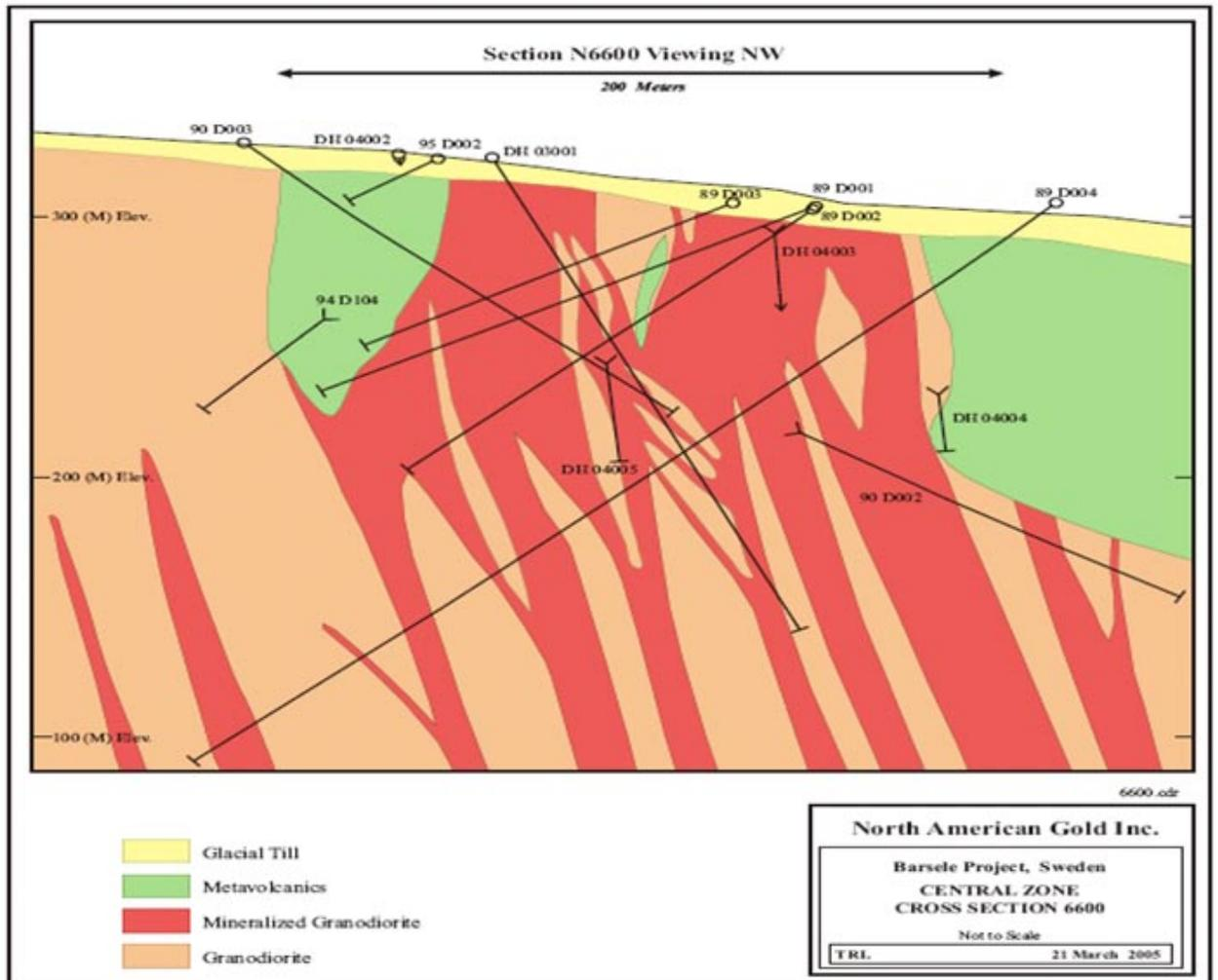
**Figure 9.1 - Central Zone Cross Section L6600N**
